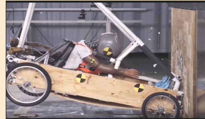
Workforce partnership with Honda: design a vehicle that would pass the major injury criteria from the National Highway Traffic Safety Administration (NHTSA) for the head, thorax, and knee of a passenger if the vehicle was involved in a 19 MPH crash.
